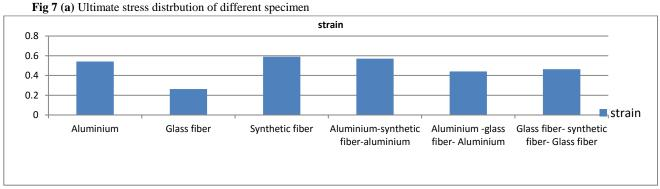
Fig 7 (b) Strain distrbution of different specimen
