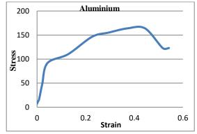
**Fig.4(b):-**Stress-Strain Diagram for Aluminum (b) Specimen-II
