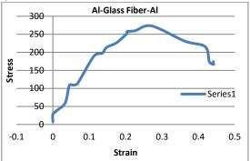
Fig.6 (b):- Stress-Strain Diagram for Synthetic Fiber Al-Glass Fiber-Al
