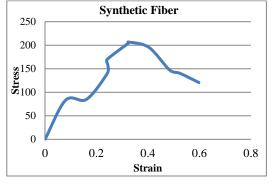
${\bf Fig.6}$  (a):- Stress-Strain Diagram for Synthetic Fiber-Al-Synthetic Fiber
