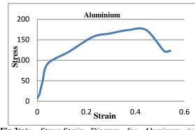
**Fig.3(a):-** Stress-Strain Diagram for Aluminum (a) Specimen-I
