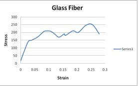
Fig. 4(b):- Stress-Strain Diagram for Glass Fiber - Specimen-II
